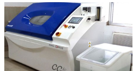
Testing machine used in carrying out the rigorous 6000-hour Cyclic Salt Spray Test
